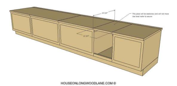
**Step 12 Directions:** Add a wood bracket (same 1x2s used for trim) on both sides of dog door entrance to brace permanent plywood piece. Use wood glue and 3/4" brad nails to secure. The 19 3/4" x 12 3/4" piece will be stationary and will not move. Use wood glue and 3/4" brad nails to secure to back edge and brackets just secured.
