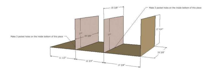
**Step 5 Directions:** Make 3 pocket holes on each of your 17" x 19 3/8" pieces so that the pocket holes are hidden inside the storage bin. The dog door entrance will be the 12 3/4" space, so make your pocket holes accordingly.
