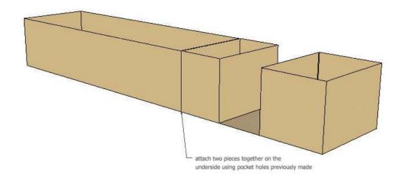
**Step 6 Directions:** Attache the two assembled pieces together on the underside and the sides using the pocket holes previously made.
