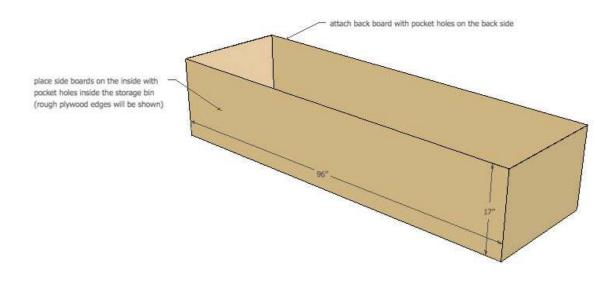
Make 4 pocket holes each on the ends of the 2 plywood sides cut at 96" x 19 3/8". Your pocket holes for the front piece will be on the inside of the storage bin. Attach the back board by making pocket holes on the backside where the wall will hide them. Flip the cube on it's side and use a brad nailer to secure the sides into the bottom piece.
